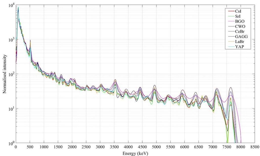
**Figure 3: Typical PGNAA induced gamma-ray spectra from the simulated scintillators.**
