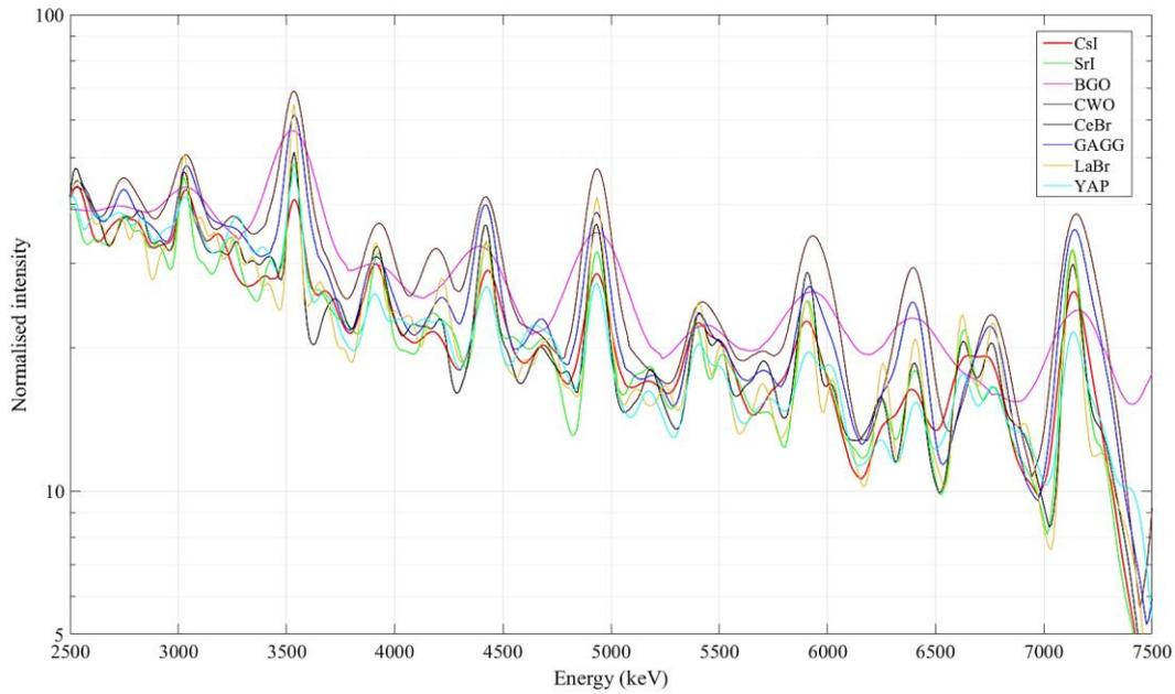
**Figure 4: Gamma-ray spectra from simulated scintillators (enlarged image of area of interest).**
