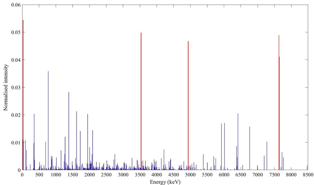
**Figure 2: Line spectrum used as an input for GEANT4 simulation. The five most intense lines in the spectrum are coloured red.**
